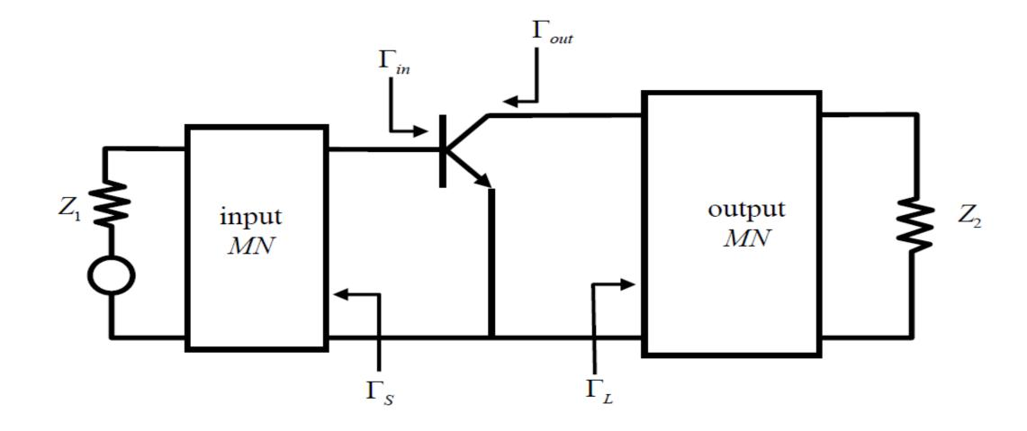
A silicon transitor has following S-matrix at 1 GHz with a  $50\Omega$  reference impedance,
