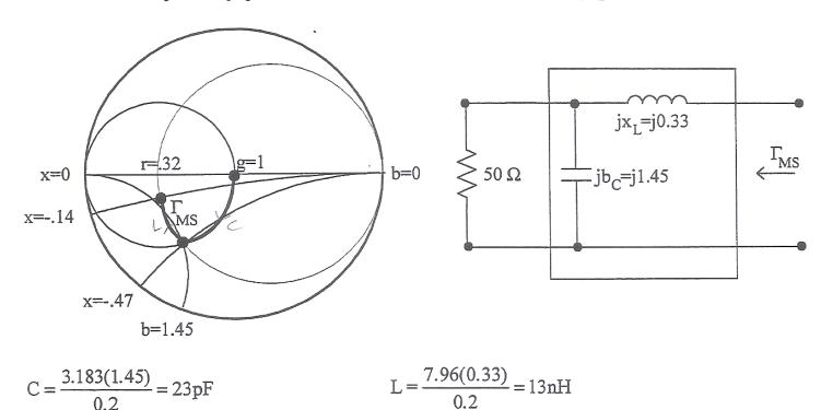
The computed load reflection coefficient,  $\Gamma_{ML} = 0.48 \angle 39^{\circ}$ . The matching output network is designed, proceeding from the 50 $\Omega$  load:
