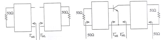
The maximum transducer power gain, under simultaneous conjugate match conditions, is obtained from the previous transducer gain formula, using  $\Gamma_{S} = \Gamma_{MS}$  and  $\Gamma_{L} = \Gamma_{ML}$
