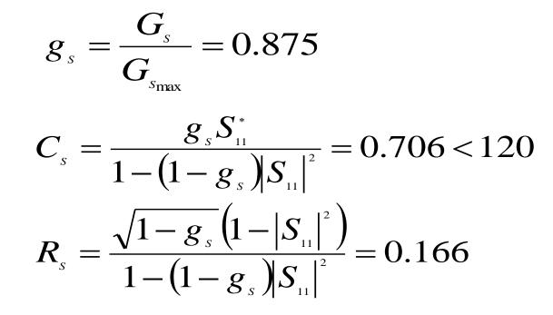
For condition 1 (output side), when  $G_L = 0$  dB:
