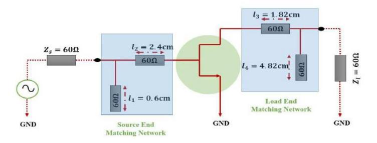
Figure 2: A transistor network with conjugate matching sections
