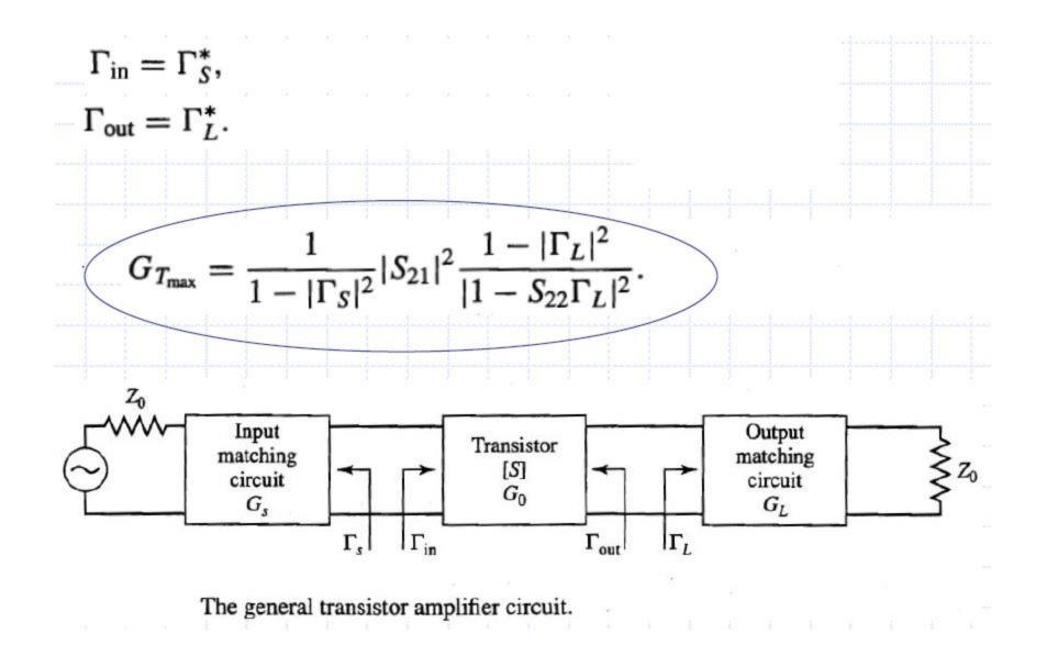
In the general case with a bilateral transistor  $(|S_{12}| \neq 0)$ ,  $\Gamma_{in}$  is affected by  $\Gamma_{out}$ , and vice versa, so that the input and output sections must be matched simultaneously. the necessary equations:
