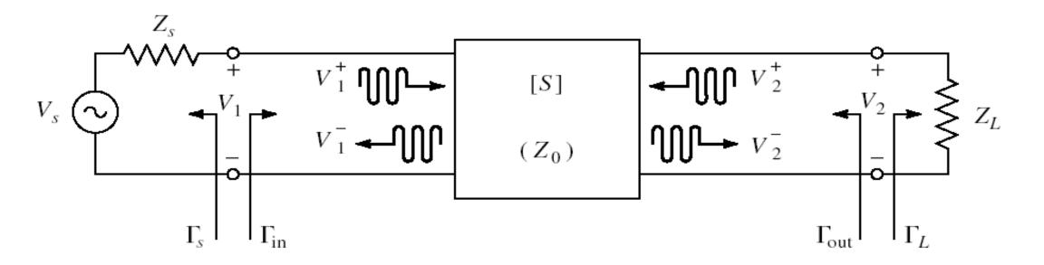
Figure 7.1: A two port network with general source and load impedance.
