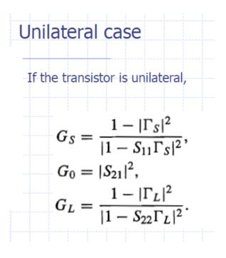
So, if you are given the S params and  $\Gamma_S, \Gamma_L$  then you can calculate the gain.
