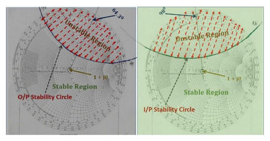
Figure 1: The stable and unstable regions for a transistor with specific S-matrix
