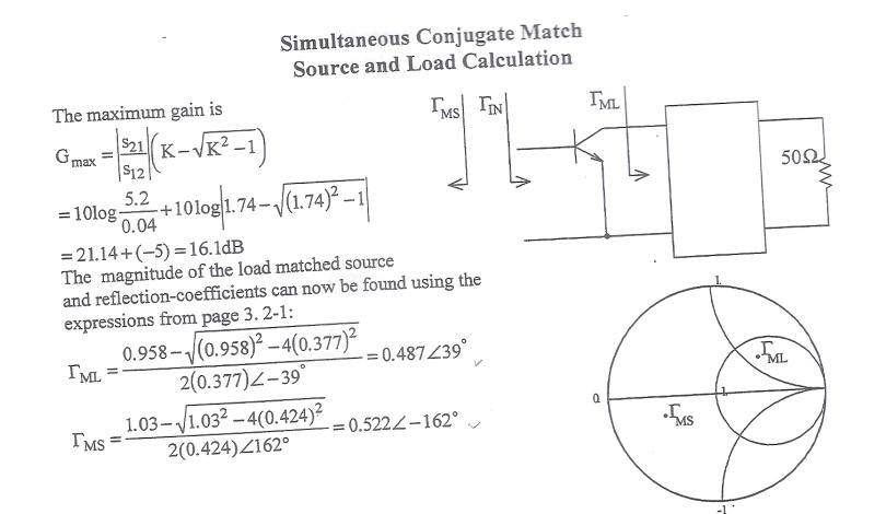
The desired source reflection coefficient,  $\Gamma_{MS} = 0.522 \angle -162^{\circ}$ . Proceeding from the 50 $\Omega$  source, the input matching network is:
