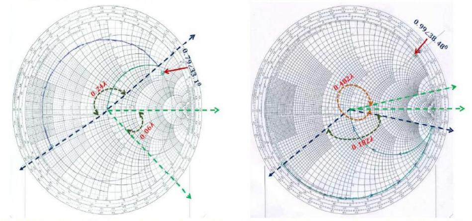
Smith Chart based solution for input matching Smith Chart based solution for output matching network network
