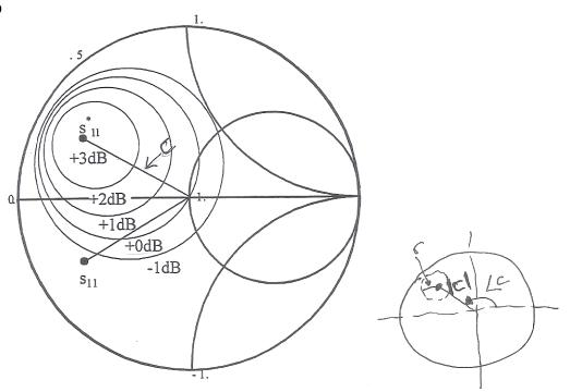
Design and amplifier with 15dB gain, using the transistor specified on the previous pages. Assume unilateral condition and find the appropriate input or output network(s).
